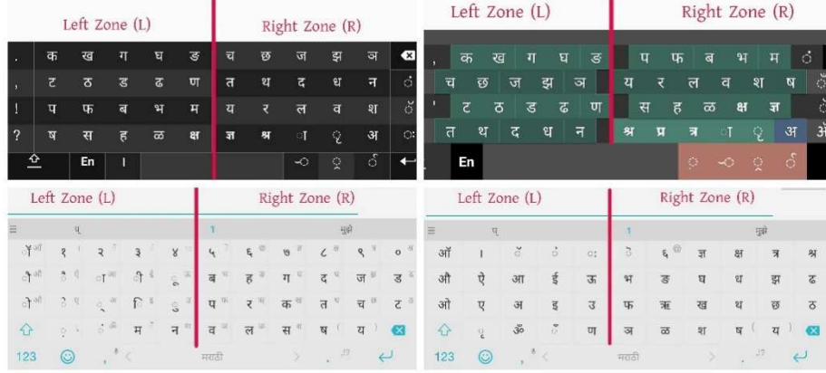
Fig. 1. Clockwise from top left, Swarachakra Non-Staggered, Swarachakra Staggered, SwiftKey Shift and SwiftKey LongPress layouts respectively.
