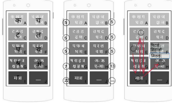
Fig. 1. (a)Shows the layout and group distribution of characters (b) shows the number of characters in each group (c) prediction bar after the swipes
